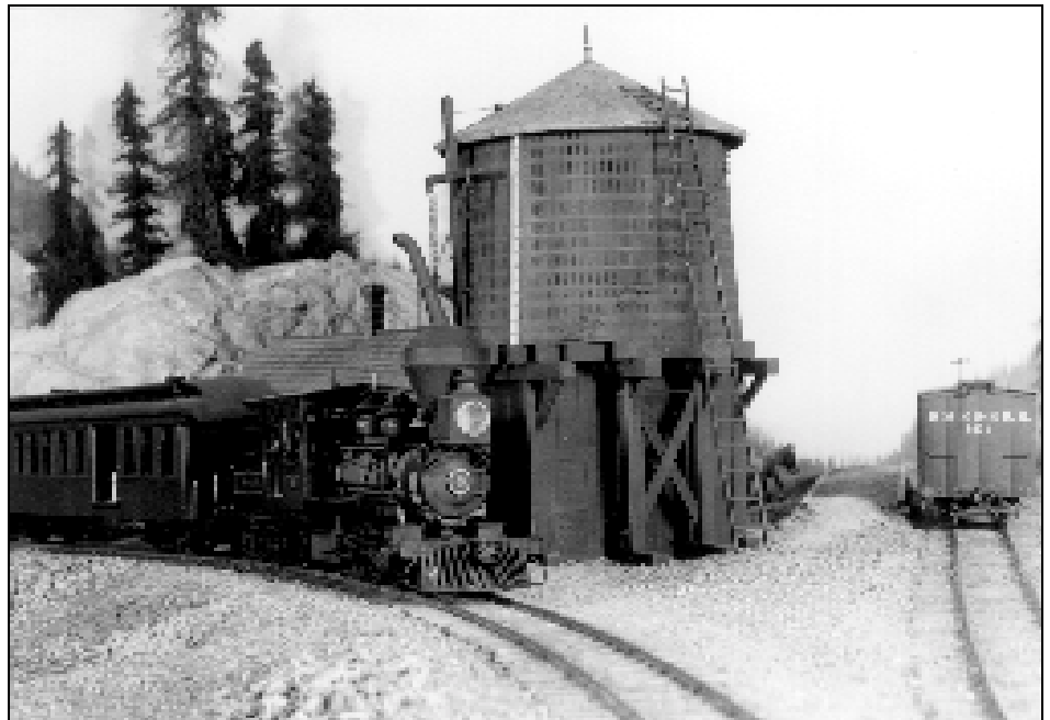
The Breckenridge mixed #279 has arrived for a water stop at Halfway, which as its name implies is halfway between Como and Boreas Pass. The water tank is a kit bashed On3 model with a redesigned enclosed base that was common in the early days of the railroad. The station/section house is scratch built of wood siding over a Plexiglas base with individual wood roof shingles.
