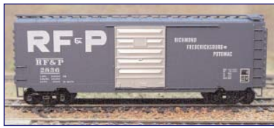
These 40' RF&P PS-1 HO-Scale box cars are Accurail bodies, custom painted by Accurail. They are blue with aluminum-colored doors, and feature prominent white lettering.
