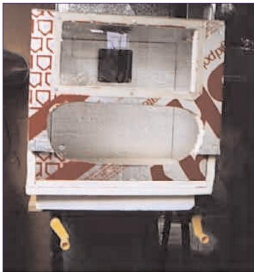
**Figure 1: The front view of a completed sand blaster, with an opening for working at the bottom and a viewing window at the top.**
