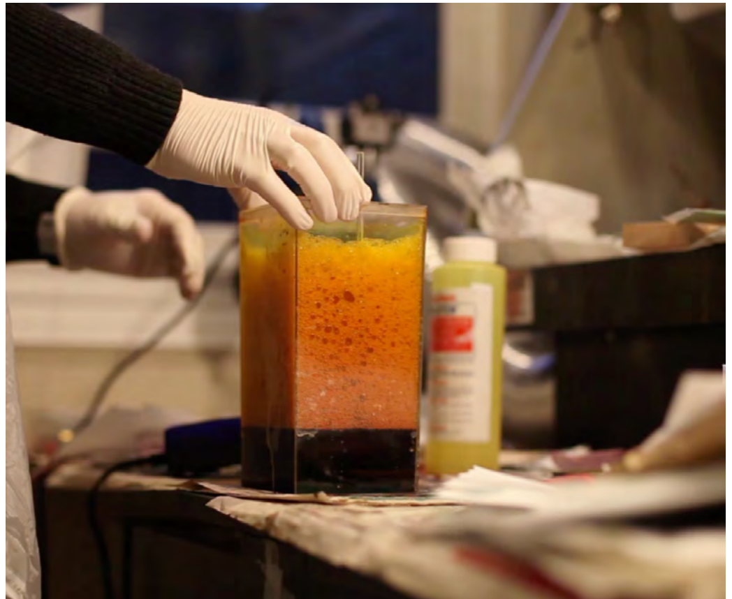
Figure 23 – The agitator bubbles air through the etchant during etching
