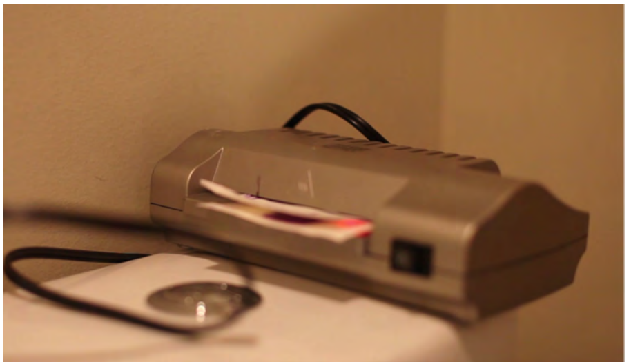
Figure 14 – Photoresist has been cut and the inner protective film removed. It is then temporarily attached to the metal with a film of water. Using the heated laminator, the photoresist is bonded to the metal.
