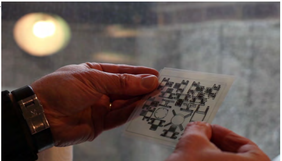
Figure 13 – The two sides of the negative need to be aligned and taped together
