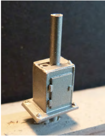
Figure 5. Relay cabinet and masts for the two-headed dwarf signal.
