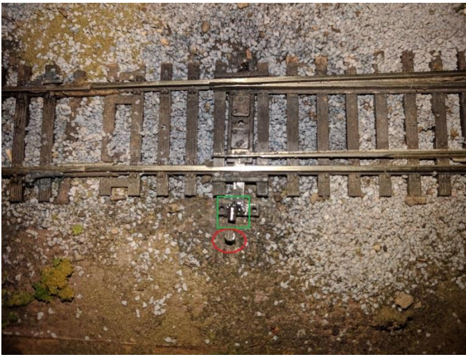
Points held in normal position with magnets.
