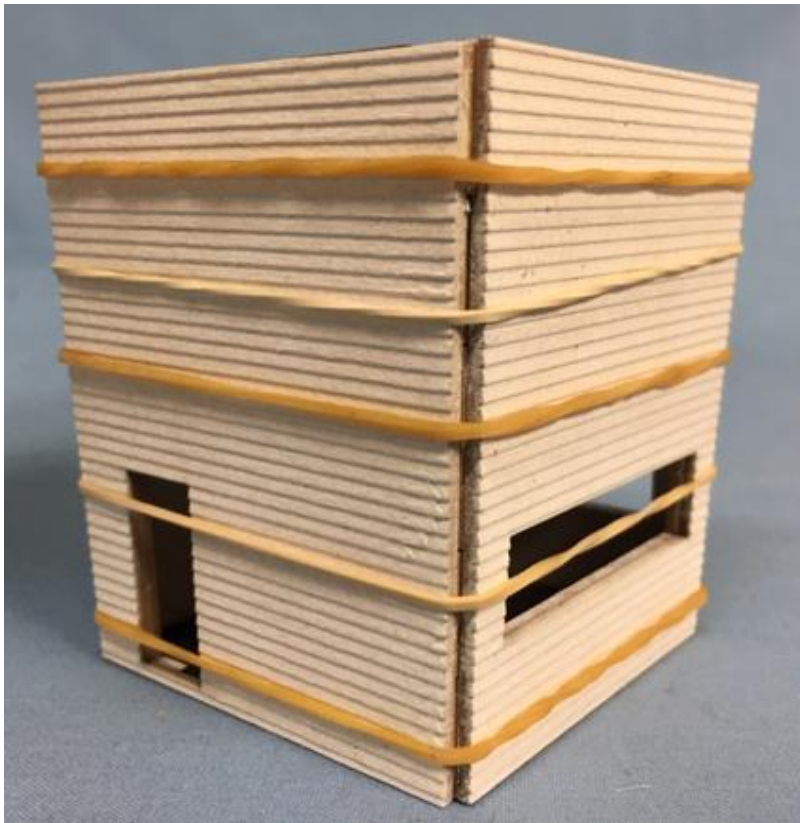
Photo 5: The inner and outer walls have been glued; the roof and floor dry fit. Rubber bands keep everything tight while the glue sets.
