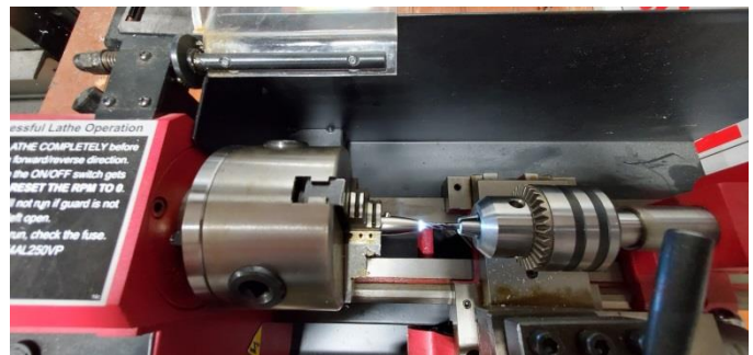
Photot 5B: Flattening and indenting the surface of the lens.
