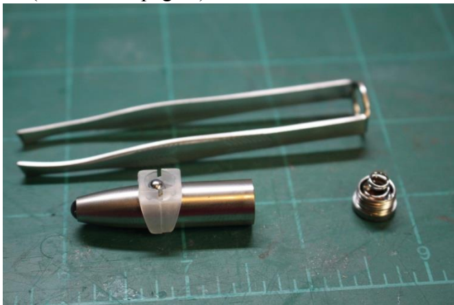
Photo 2: Disassembly is easy. The end cap unscrews for access to the supplied batteries
