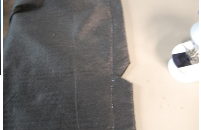
Photo 8: Cut notches in the hem to allow clearance over the eyebolt “hooks”. This can be done after the skirts are hung, but it is easier to do before installing them.
