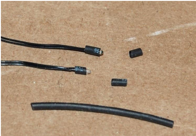
Photo 16: 2 mm shrink wrap tubing
