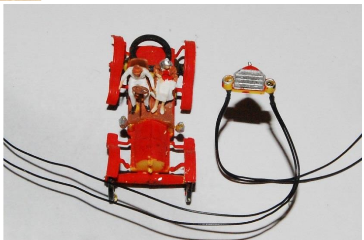
Photo 19: Bulbs glued to radiator/headlamp assembly.
