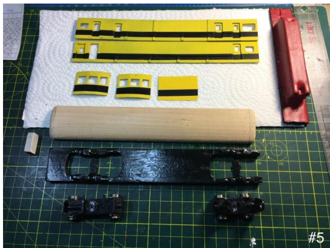
Photo 4: This is the model out of the paint shop before it received the black stripe. Notice the weight. As the frame is soft pine, I needed extra weight for traction effort.
