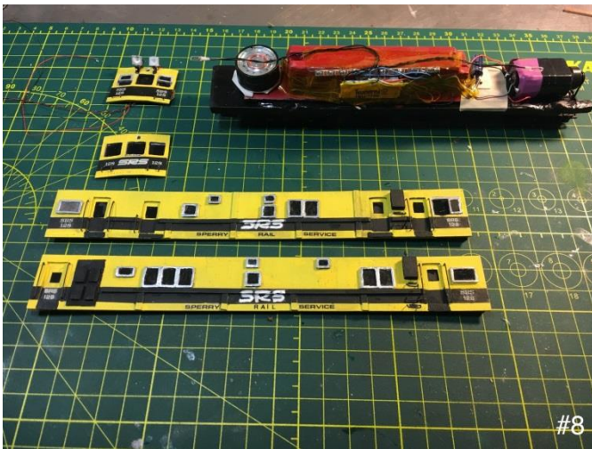
Photo 7: This picture shows the decoder and micro-LED for scratchbuilt flood lights. There is also a homemade terminal block for all decoder wiring.
