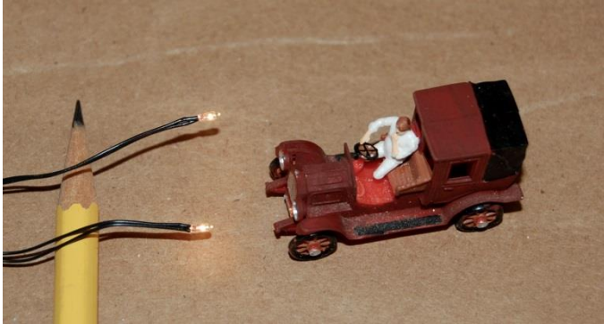
Photo 3: Circuitron 1.5 volt bulbs)
