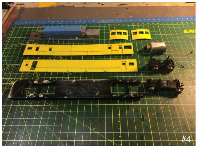
Photo 4: This is the model out of the paint shop before it received the black stripe. Notice the weight. As the frame is soft pine, I needed extra weight for traction effort.
