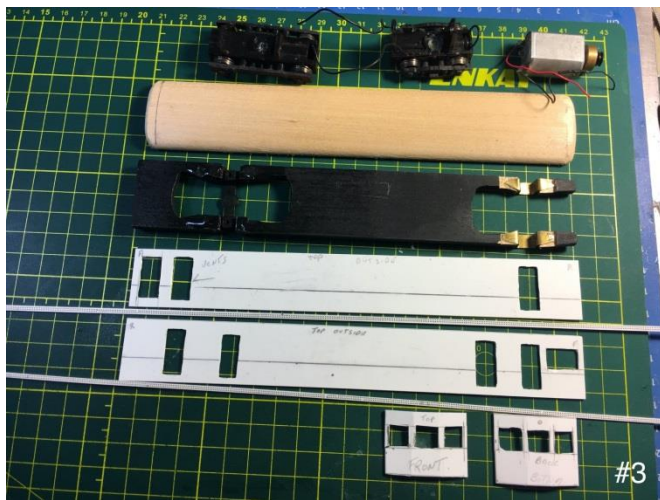
Photo 3: This photo shows the major components. Note, the frame has been cut out and body bolsters have been applied.
