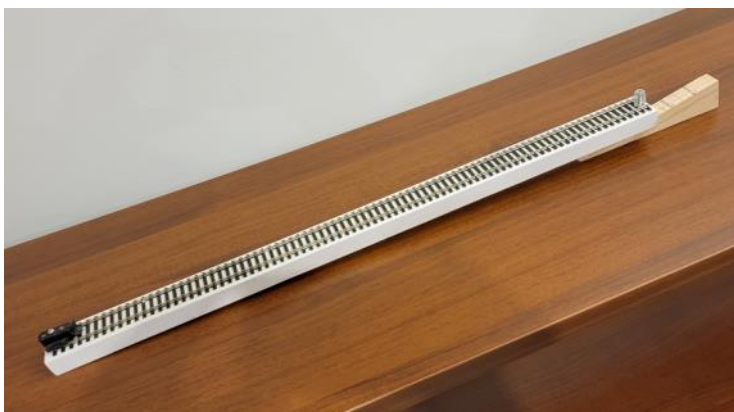
Photo 19 - Test Track with Kadee Coupler Gauge and wedge to adjust slope.
