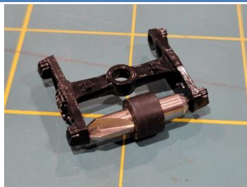
Photo 10 - Using Tuner to Improve Socket for Axle.
