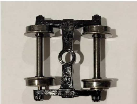
Photo 14 - Wheelset on right is centered by washers. Wheelset on left is loose and off center.
