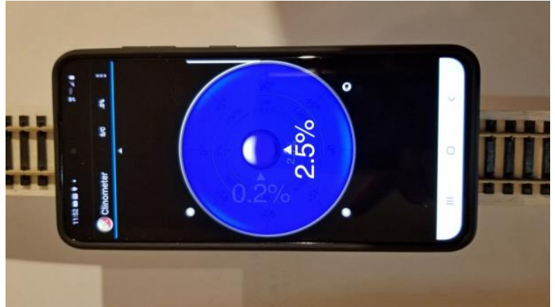
Photo 6 - Clinometer App Measuring 2.5% Grade.
