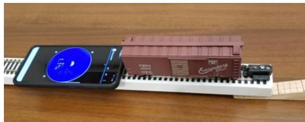
Photo 20 - The completed car on the test track. Coupler height matched and ready to roll on a 1.1% grade.
