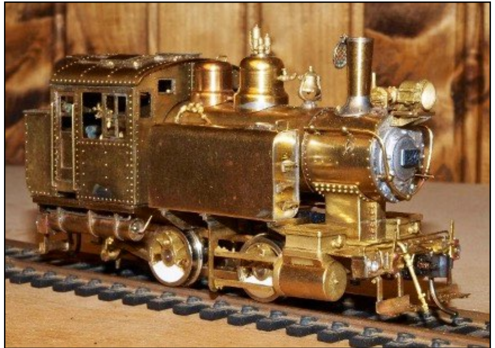
Photo 11: I turned the domes and stack of this tank engine on my drill press using needle files. The sir tanks under the cab are scratchbuilt from brass tubing.
