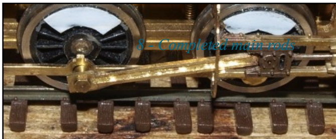
8 - Finished main rods
