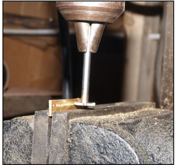
7 - Cutting main rods.
