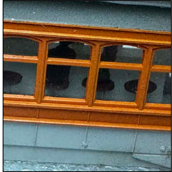
5 - Stools were made with discs of styrene supported on thin brass rods.
