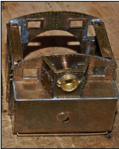
Photo 10: I used brass angles to hold the front, rear, and side walls together – Solder all connections.
