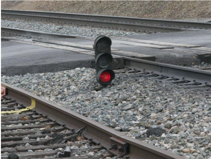
Photo-5 – A dwarf signal on the old C&O had a light arrangement of Y/G/R and indicated a slow speed. Y/R on the same dwarf is Approach Slow, Y is Restricting.
