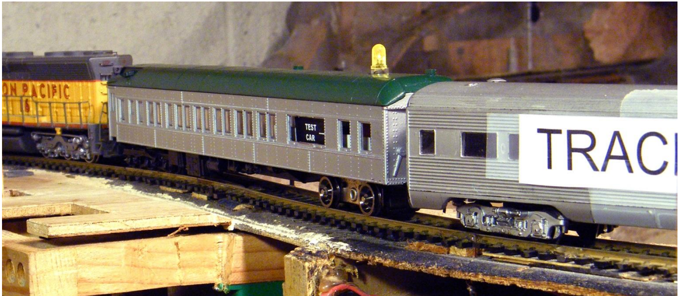
Figure 1 - Track Test Train - A track test train traverses a tricky piece of track consisting of an “S” curve, a wye switch, and a convex vertical curve. Testing is being done during the track laying stage and scenery will be added only after the track is certified as reliable. Note the wooden shims under the ties used to adjust the vertical contour of the track.
