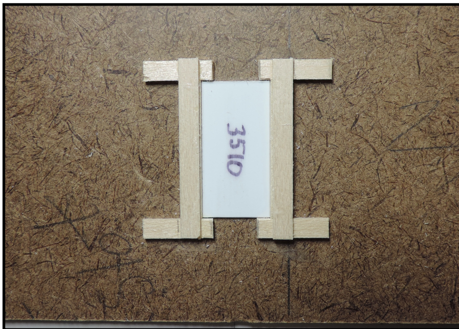
Photo 2 – Window Jig with the styrene blank used to trace the wall openings to be cut.
