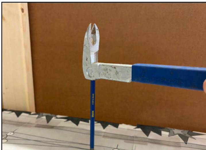
Photo 5 – I used an awl and a tack hammer to punch holes on the track centerline every few inches through the paper plan onto the plywood. I also marked the ends of turnouts for proper alignment later.
