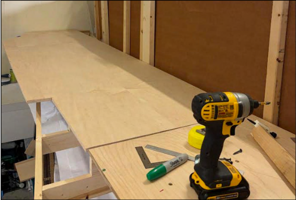
Photo 4 – the final shape of the port has been cut out. Note the squared off section to the lower left with benchwork dropped down below it. This will be the river level and gives room in front of the relocated bulk facilities for a prototypically accurate sized ship model ~4 feet in length.
